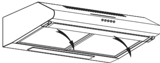
6. To change the light, press the lamp cup, take out the bulb counter-clockwise.
