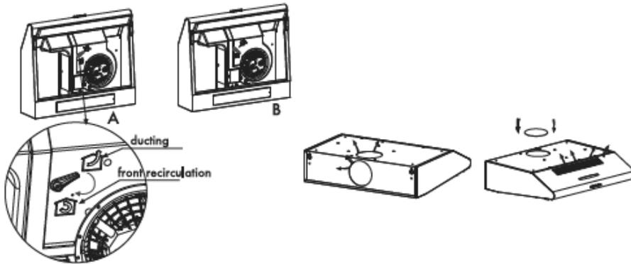
When you choose “front re-circulation mode”, the charcoal filter must be installed.
